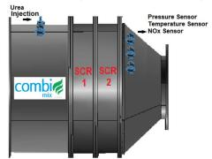
Although sulfur is not a poison to conventional SCR catalysts at low temperatures, ammonia and sulfuric acid condenses as liquid ammonium bisulfate NH4HSO4, (ABS) in the catalyst pore structure, which inhibits the catalysts performance. ABS may also adversely affect engine operation by increasing exhaust backpressure. The condensation reaction for ammonium bisulfate formation is written as:
