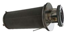
The PMF operating procedure of particulate reduction takes place by the exhaust gas passing through the external wall of the filter where the soot is captured. The gas then passes into the internal chamber then exits the system.
